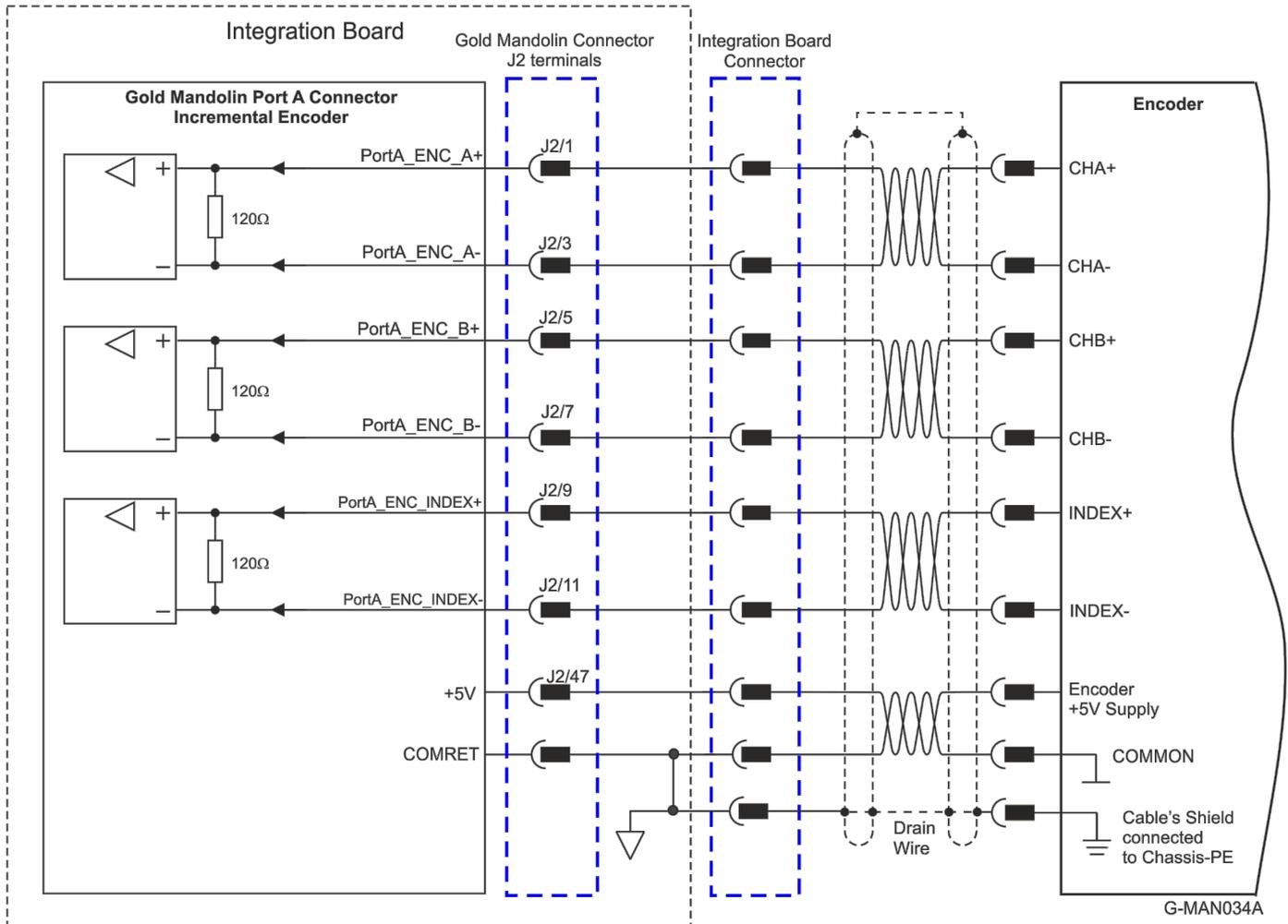
Figure 15: Port A Incremental Encoder Input – Recommended Connection Diagram
