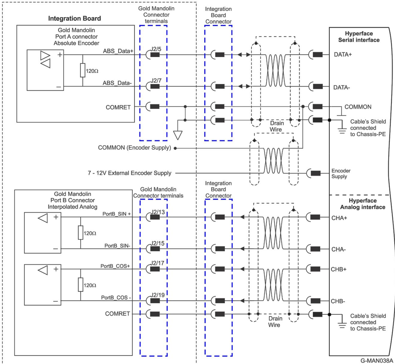
Figure 19: Absolute Serial Encoder – Recommended Connection Diagram for Stegmann Hiperface
