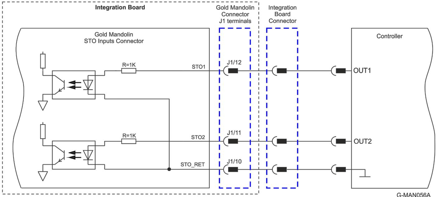
Figure 32: STO Input Connection – TTL Option
