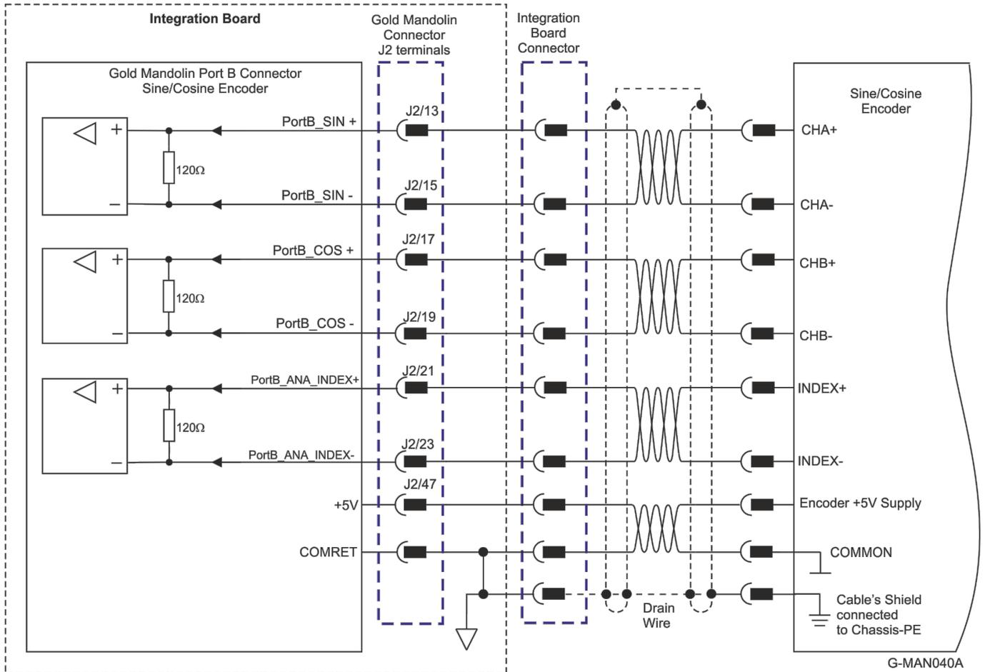
Figure 21: Port B - Interpolated Analog Encoder Connection Diagram
