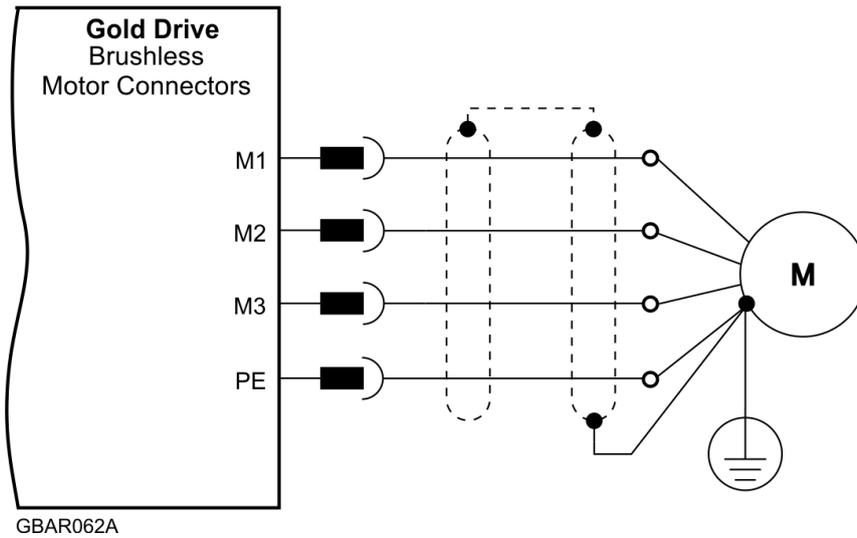
Figure 6: Brushless Motor Power Connection Diagram
